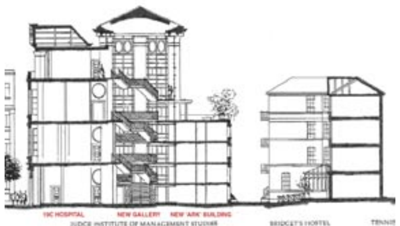
The Ark block had to be compressed vertically to also allow light to its neighbour across a narrow alley. This also lets Eastern side-light into the Gallery, which warms it in the winter. Light-shelves up this wall prevent summer heating.
